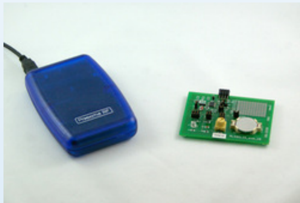
DVK90129 kit including a Proxima RF Desktop reader and Melexis EVB90129
